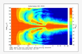
The CF210 is a vertically stacked design with dual 10" drives that provide extended vertical control of plus minus 45 degrees from 500 hz onwards,
