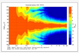
The horn offers smooth 60° horizontal coverage with no hot spots, ensuring controlled dispersion.
