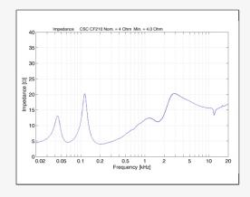
Dual 4-ohm components maintain amplifier compatibility with bi-amp operation or passive full-range use.
